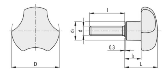
$\begin{array}{lll} D & = 40 \\ \text{d1} & = 16 \\ Dg & = - \\ \text{I2} & = 13.5 \\ L & = 27 \\ \text{L1} & = 40 \\ \text{Weight in (g)} & = 36 \\ \end{array}$
